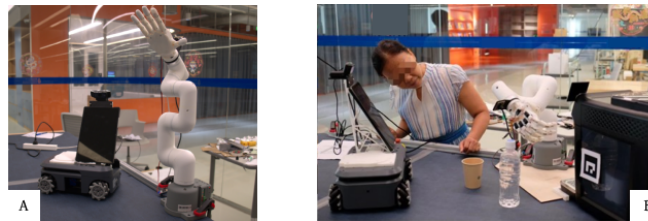
Figure 4: The prototype photos. To ensure participants’ safety and better robot movement accuracy for a smooth experience, the robotic arm is fixed on the table. A: Photo of the prototype with the robotic arm fixed on the table. B: How participants use prototypes.
